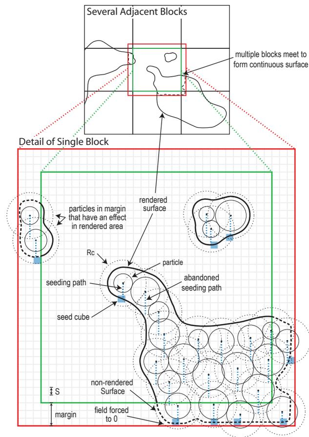
**Figure 2:** 2D illustration of block subdivision. The green box contains the polygonized surface and red box outlines the margin.
