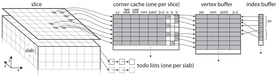
**Figure 3:** Data structures used in the Marching Slabs algorithm.
