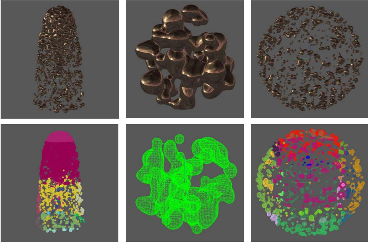
**Figure 6:** Screenshots of simulations used for performance comparison. Top row from left to right: fountain, blob, and explosion simulations. Bottom row: wireframe views of simulation with blocks identified by different colors.
